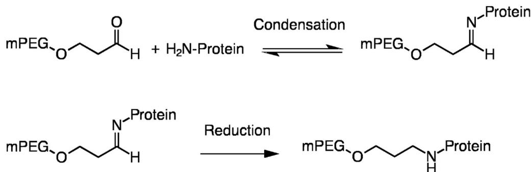
**Figure 19.** Two-step PEGylation by aldehyde chemistry: first step: formation of a labile Schiff base; second step: reduction of Schiff base to a stable secondary amine.
