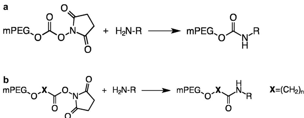
**Figure 8.** PEGylation of primary amines in proteins (H<sub>2</sub>N-R) leading to formation of (a) carbamate and/or urethane linkage or (b) amide linkage.
