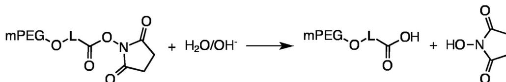
**Figure 9.** Hydrolysis reaction of N-hydroxysuccinimide-activated PEG reagents yielding the corresponding PEG acid and N-hydroxysuccinimide (L: linker group between PEG and active N-hydroxysuccinimide head group).
