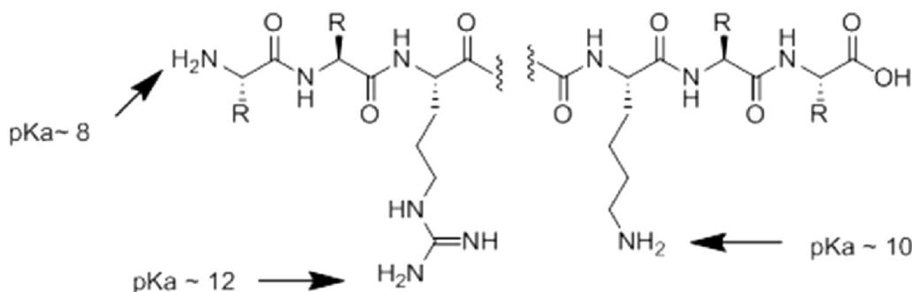
**Figure 18.** Differences in pKa of N terminal amine versus the  $\epsilon$  amino acid side chains allows site-directed PEGylation controlled by pH.
